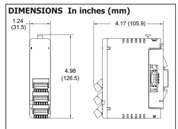
Controller Series' high density packaging and DIN rail mounting saves time and panel space. The backplane connection provides power and communication to the module and snaps easily onto standard top hat (T) profile DIN rail.
